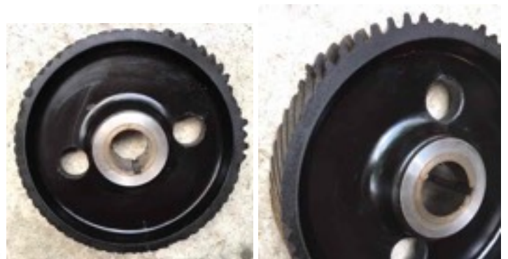
My fibre cam gear - with most of the teeth chewed off
